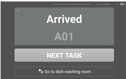
6. The “Arrived at task point” interface is the same as the “Call arrival” interface, the user needs to judge whether the next task can be performed or return directly based on the remaining space of the robot currently loaded
