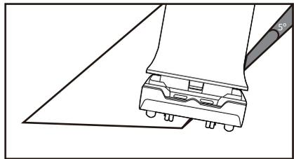
The gradient recommended for carrying dishes should be within  $5^\circ$  and not exceed  $7.5^\circ$  at most
